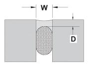
EXPANSION JOINTS - The minimum width and depth of any sealant application should be 1/4" by 1/4" (6mm by 6mm). The depth (D) of sealant may be equal to the width (W) of joints that are less than 1/2" wide. For joints ranging from 1/2" to 1" (13mm to 25mm) wide, the sealant depth should be approximately one-half of the joint width.
